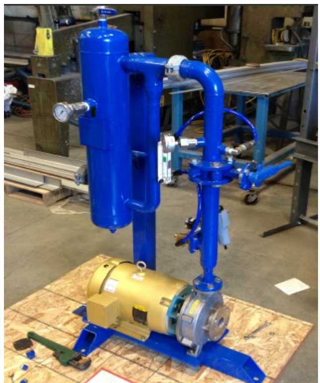
Proposed DAF Aeration Unit
